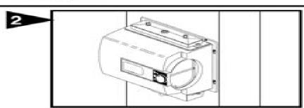
Center punch the four side mounting holes on the template and drill with an 1/8" drill bit. Insert four sheet metal screws in the side mounting holes until the heads project about 3/8". Hang humidifier from the four screws and install drain pan, evaporator pad and distributor trough. Adjust humidifier until level and tighten four screws. Remark four remaining holes if necessary. Remove humidifier and drill four remaining holes.
