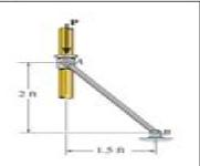
Internal Loading: The normal force developed in rod AB can be determined by considering the equilibrium of collar A with reference to its free-body diagram. Fig. a.
