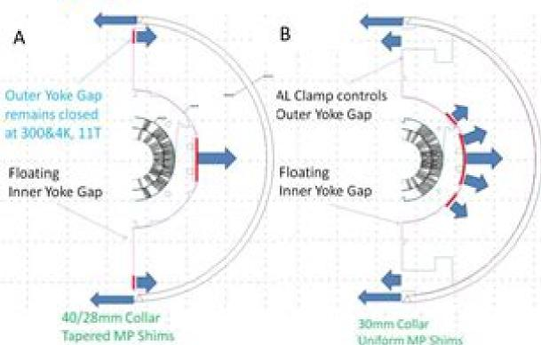
The 30-mm horizontal collar width is virtually the maximum possible in the available space between the two coils in the double-aperture configuration with two independent collared coils.
