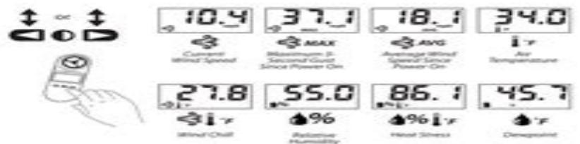
4) Select the units of measure. Press ► while holding ● to scroll through the units of measure.
