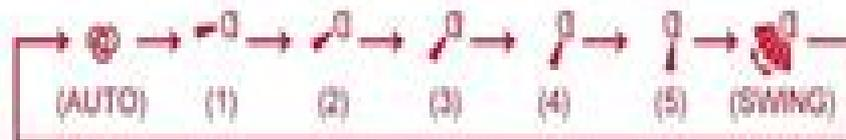
(AUTO).....The vane is set to the most efficient airflow direction. COOL/ DRY/FAN:horizontal position. HEAT:position (4).
