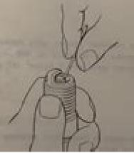
Remove carbon deposits with plug cleaner or wire brush.
