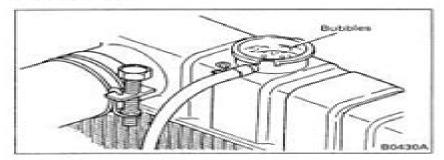
Remove the pressure cap from the radiator, and run the engine to raise the coolant temperature up to around 90°C.
