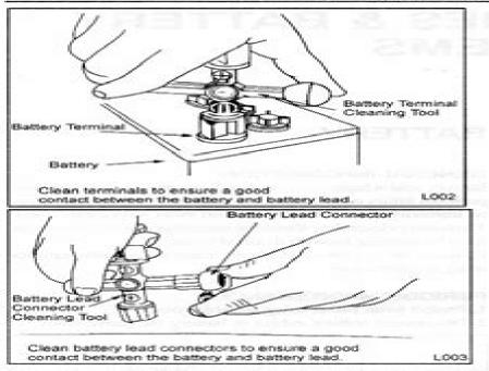
scrubbing area with a stiff brush, taking care to avoid spreading corrosion residue, and flush area with clean water.
