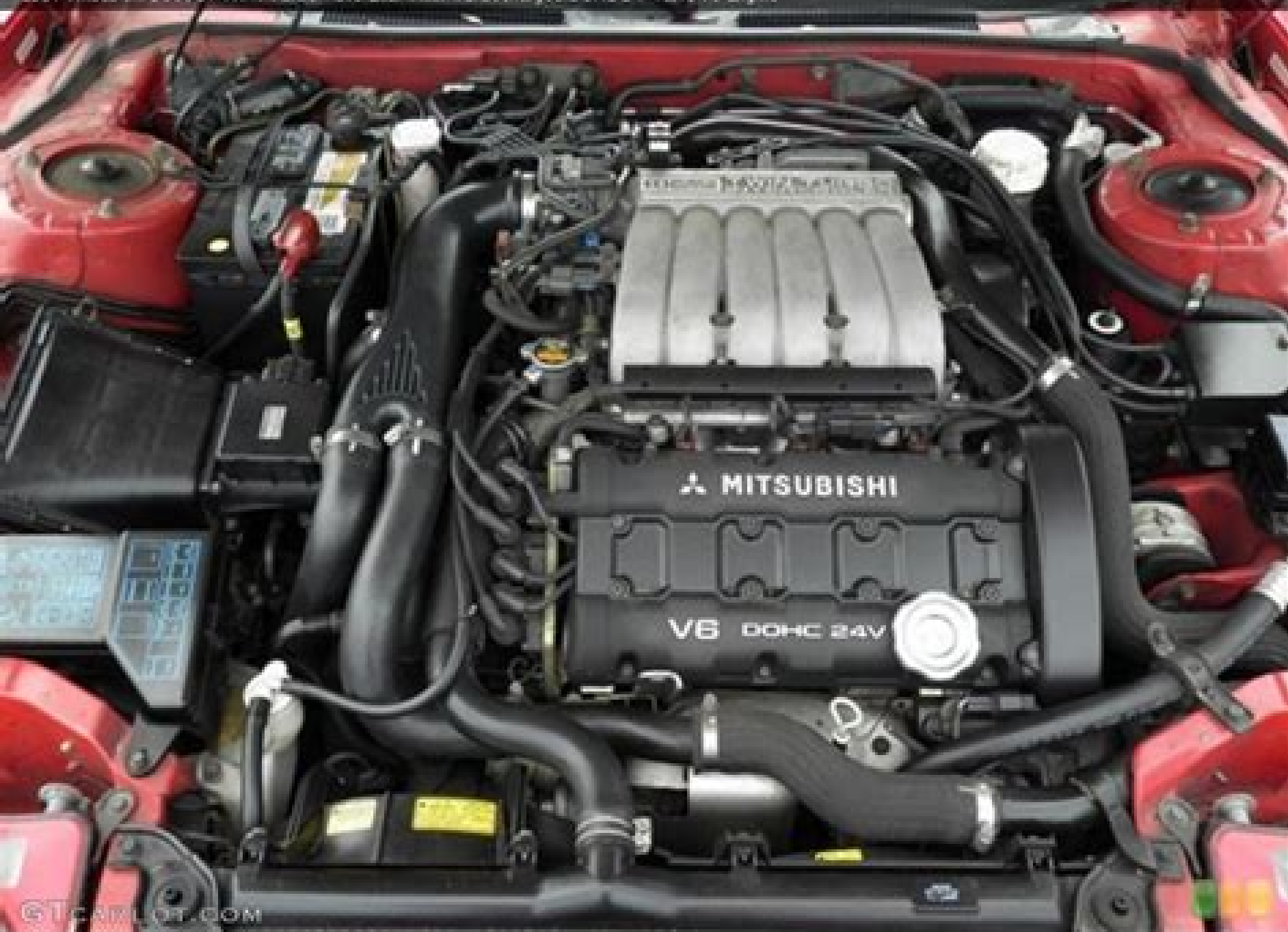
1997 Mitsubishi 3000GT VR-4 Turbo - 3.0 Liter Twin-Turbocharged DOHC 24-Valve V6 Engine
