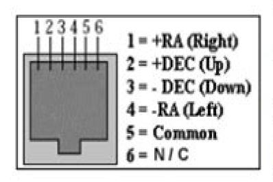
The Left, Down, Up and Right signals are driven from optically isolated photo transistors that conduct when telescope movement is desired. They can sink up to
