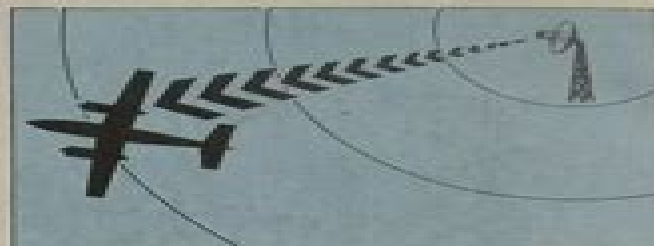
Ground radar sweep "interrogates" aircraft at 10-15 second intervals.
