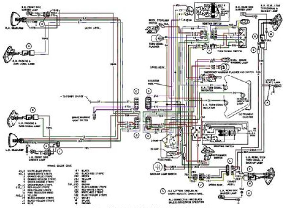
Wiring diagram for the exterior lights and turn signals—1970 Broncos
