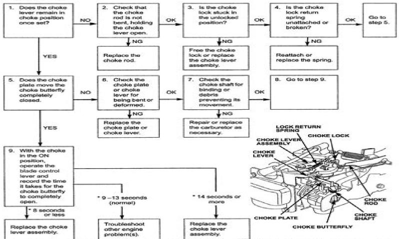
The choke base contains the damper device that controls the opening speed of the choke butterfly. The damper is ambient temperature sensitive. Times were calculated at 70°F. Your time may vary slightly, based on the ambient temperature. The colder the ambient temperature, the longer it will take for the choke to fully open.
