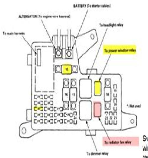
Swap the radiator fan relay with the power window relay to test. But, replace back radiator fan relay to avoid overheating.
