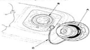
is the fuel fill cap seal missing or damaged, is the fuel fill pipe damaged, or is the lether cord caught under the cap?
