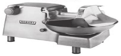
The Model 84186 Food Cutter is designed to cut and mix a wide variety of products. With products in the rotating 18" stainless steel bowl, rotating knives cut and mix them inside the bowl cover. The food cutter is powered by a 1 horsepower motor and is available for single- or three-phase electrical service.
