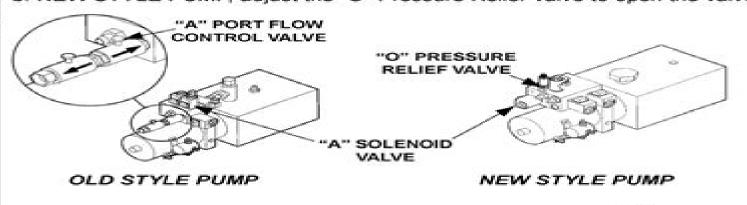
Check the "A" Solenoid Valve Coil for power.
