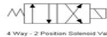
4 Way - 2 Position Solenoid Valve
