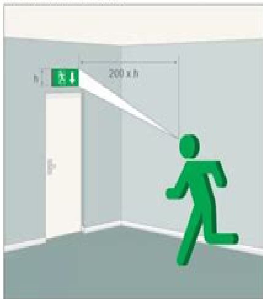
Internally illuminated signs - 200 \times the panel height
