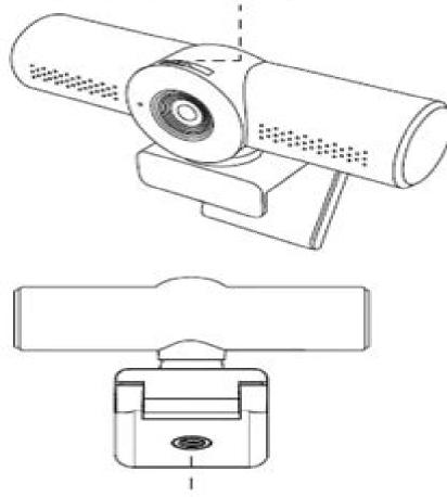
Tripod thread for ¼ inch screw (Tripod not provided)
