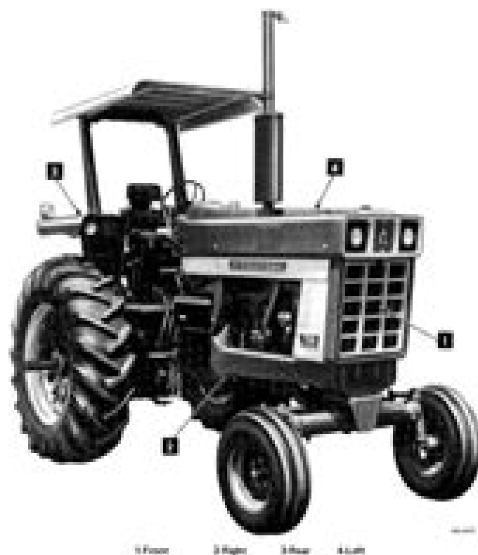
Illustr. 2 Right side of tractor showing terms of location.
