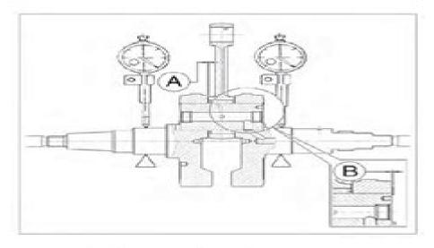
Check the connecting rod side float into the flywheels. It must be 0,4+0,5 mm (0.0157+0.0197 in).
