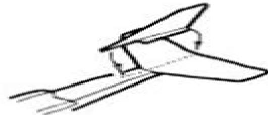
**9** Glue the rudder to the center of the stabilizer and the top of the fuselage. Take care to get it straight.
