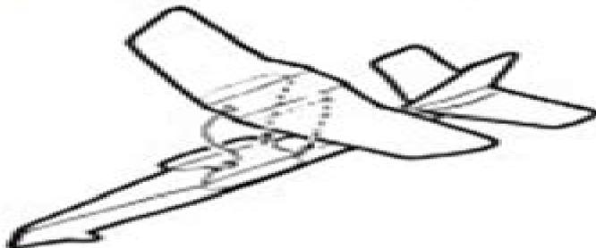
**10** Glue the wing to the top of the fuselage. The front edge is tucked and glued under the triangular tab at the back of part 10. The rear edge floats a bit at the back.
