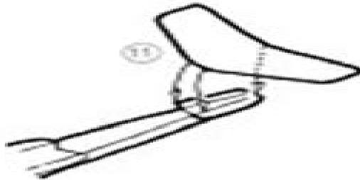
**8** Glue stabilizer 11 to the tabs at the rear of the fuselage. Make sure it is straight.
