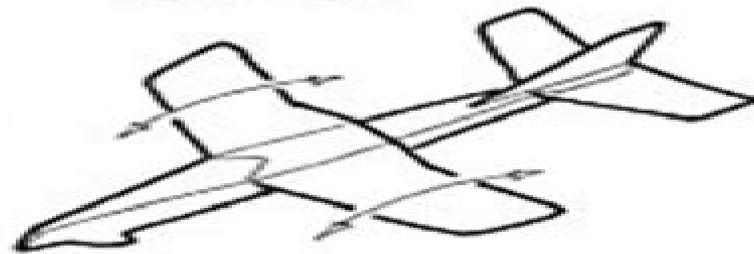
**11** Add a bit of camber (front to back arching) to the wings, let it dry a bit, and you are ready for test flights.
