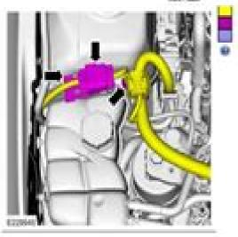
Remove the tost and position the degas bottle seale. Detach the costant hose retainer.
