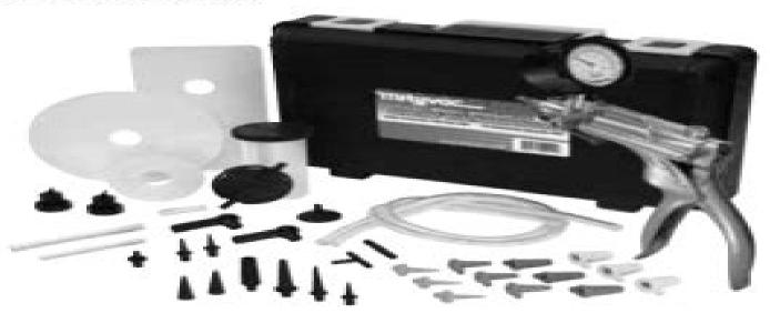
CAUTION: Never exceed the rated pressure of the gauge, as this can cause loss of accuracy and permanent damage.
