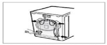
Unscrew the 4 boils with the wrench supplied.
