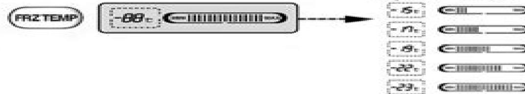
**How to adjust the temperature in the refrigerator compartment**
