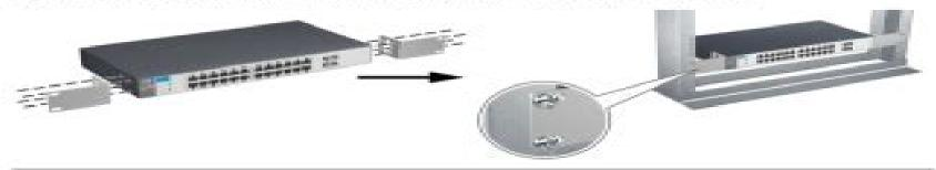
Table or Desktop Mounting: Attach the four selfadhesive pads (included in the accessory kit) to the bottom corners of the switch.
