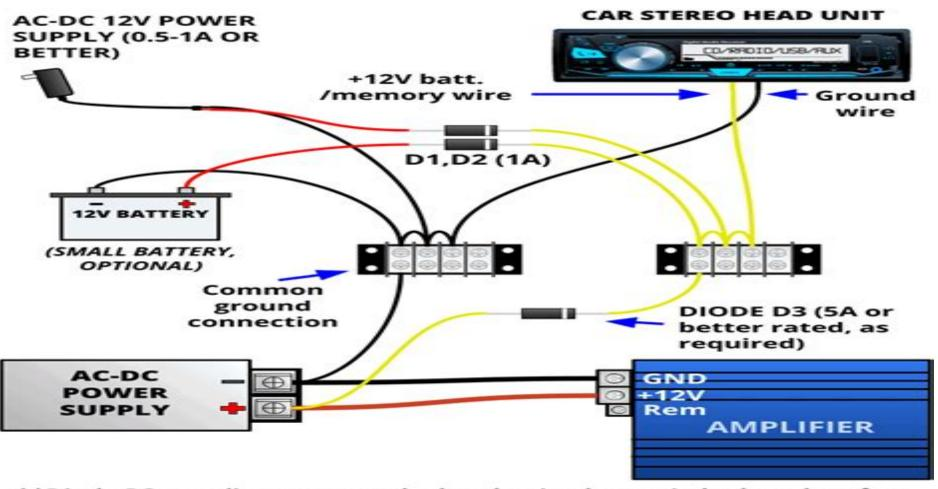
\*\*Diode D3 supplies power to the head unit when switched on therefore should be rated for the head unit's maximum current draw. Optionally, you can also use multiple diodes in parallel instead of a single diode of higher current rating if they add up to the same or more.
