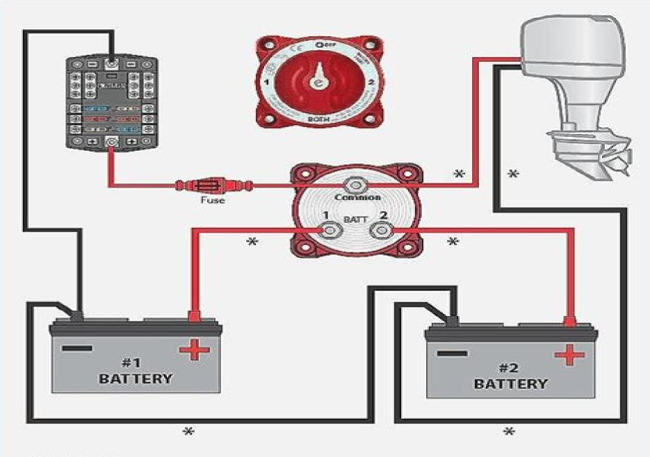
All cables marked with an \* are sized for starting the motor
