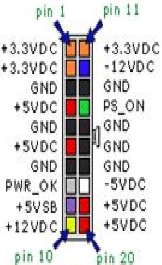
ATX 20 pin Molex Main Power Connector
