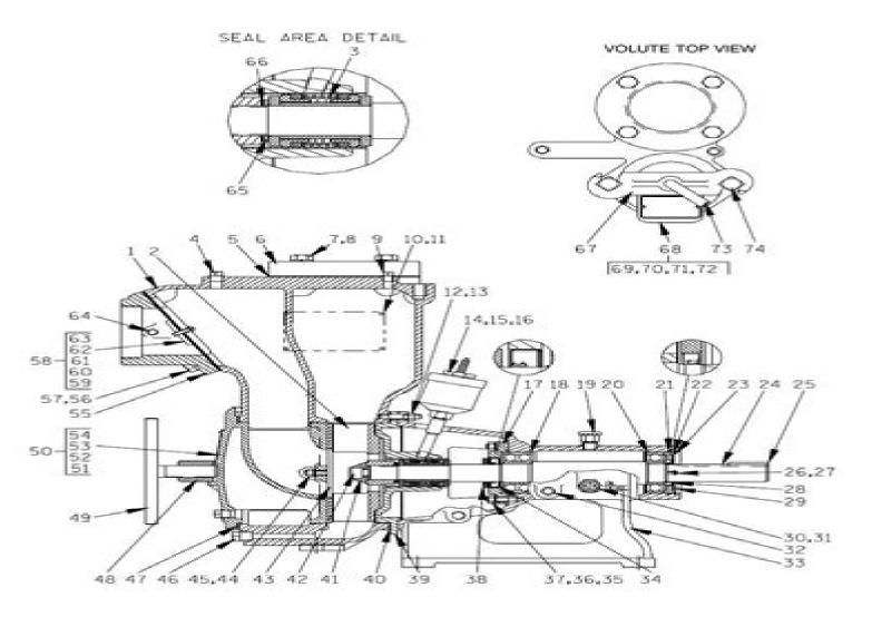
Figure E-1. Pump Model 14A2-B
