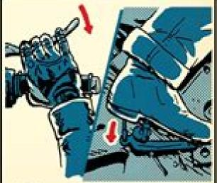
Bring yourself to a stop by using the front and rear brakes in tandem.
