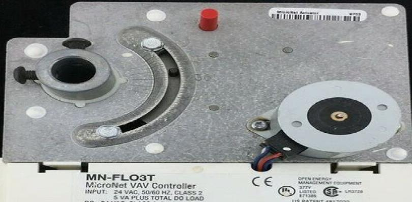
DO: 24 VAC, CLASS 2, PILOT DUTY DO1 + DO2: 24 VA TOTAL LOAD DO3: 12 VA
