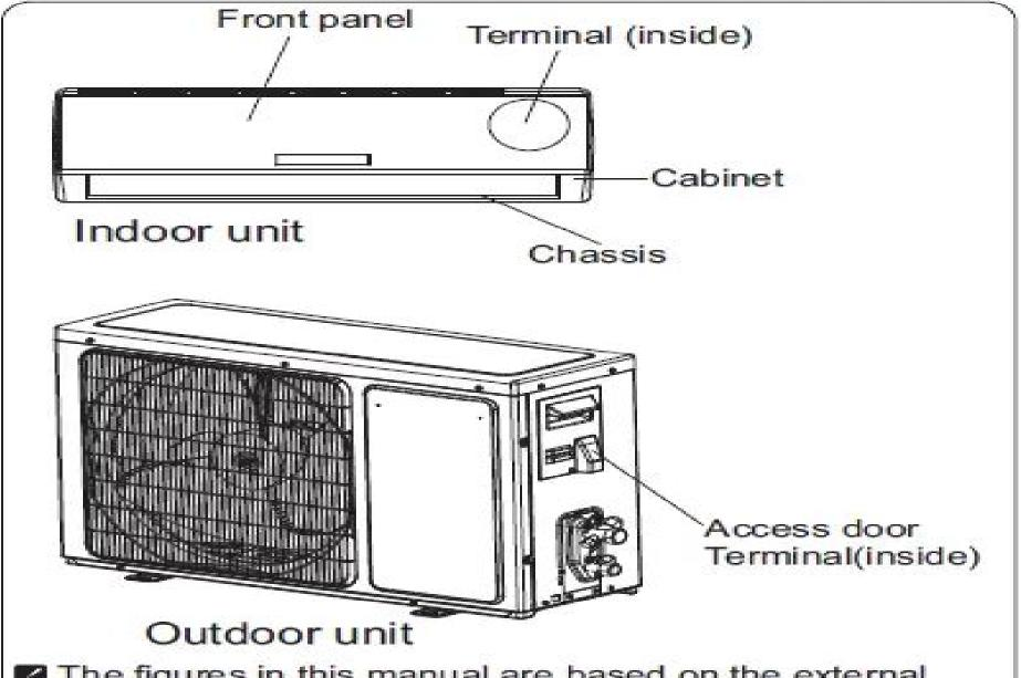
The figures in this manual are based on the external view of a standard model. Consequently, the shape may differ from that of the air conditioner you have selected.
