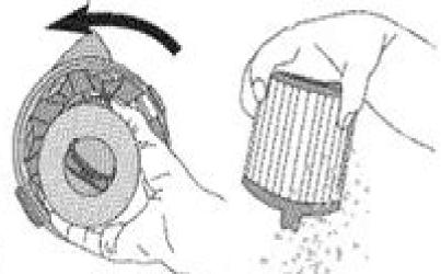
Grasp filter and twist to remove from lid. Shake dust from filter.
