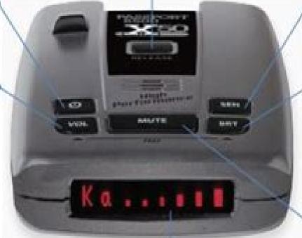
Press to adjust detector sensitivity (Highway, Auto, Auto NoX)
