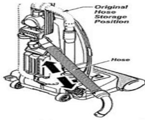
Re-insert the hose into the original storage position from which it was removed. Press firmly to assure connection. Rotate hose release lever clockwise to the locked position.
