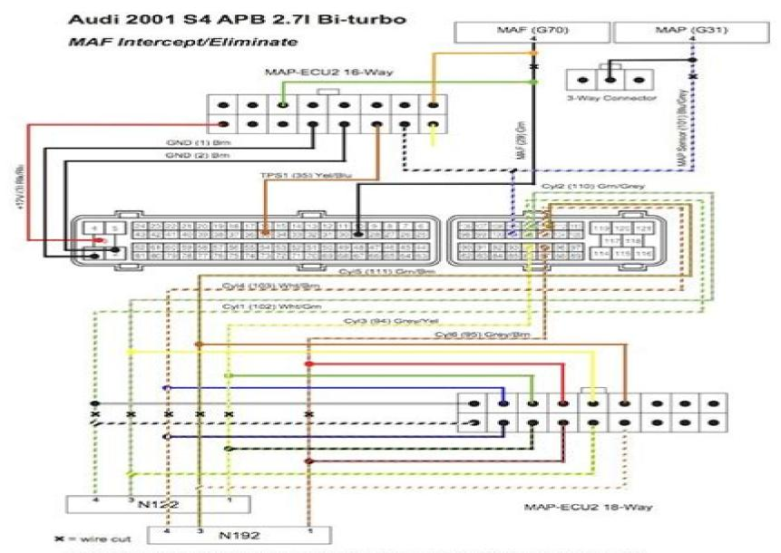
Note: Configure to 6-Cylinder Coil on Plug, MAF Intercept - MAP Y-Axis, Ext MAP = FCD1, Analog 2 Output = FCD1 for fuel cut defeat (if required). Firing Order: 1-4-3-6-2-5
