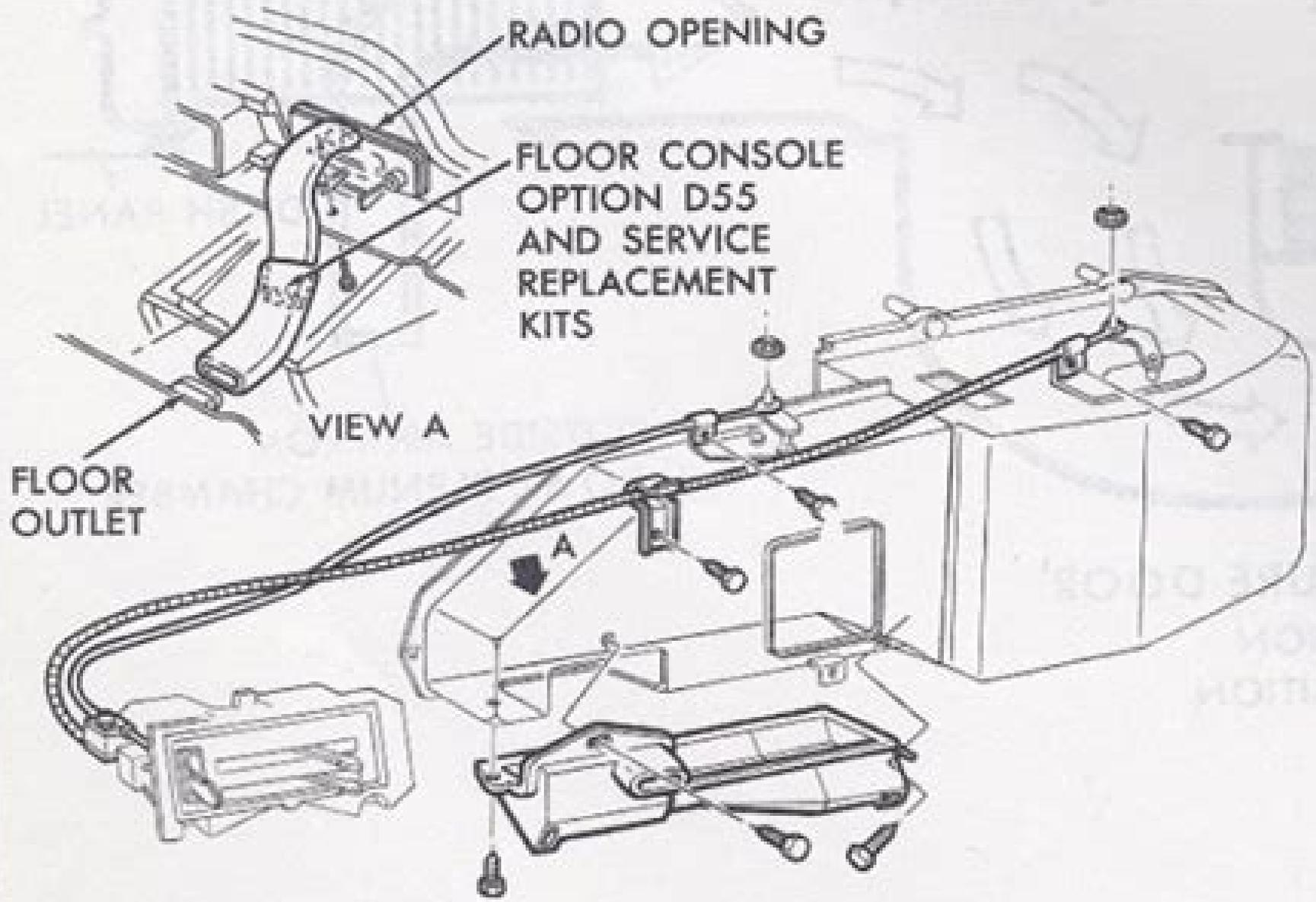
Fig. 3—Heater and Air Distributor
