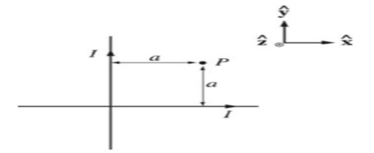
Consider two very long, straight, insulated wires oriented at right angles. The wires carry currents of equal magnitude I in the directions shown in the figure above. What is the net magnetic field at point P?
