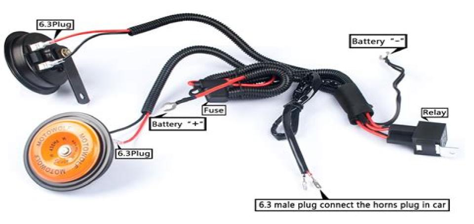
Connection diagram for the horns wiring harness System
