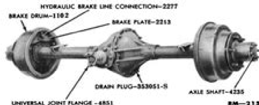
Figure 1— Standard Rear Axle Assembly
