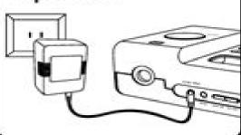
Attach AC adaptor cable to jack on back of the iH8 and plug the other end into a wall socket.
