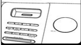
Press the Radio button and press again to select AM/FM band. Turn the Set Wheel to tune in a station. Press and hold a preset button (1, 2,3 or 4) to save the station as a preset.
