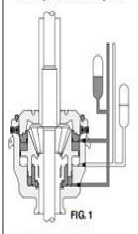
SECONDARY CHAMBER connected to CLOSING CHAMBER (S - C)
