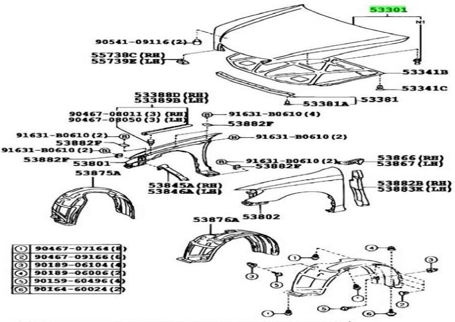
N 1 This part is not supplied as an individual part, because it is hard to assemble / disassemble due to the structure
