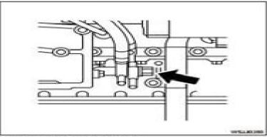
8. Remove the engine foot.
