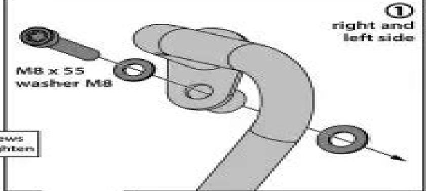
! Insert screws do not tighten
