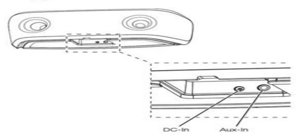
If you are going to use your JBL OnBeat aWake with another audio source, plug one end of a 3.5mm (1/8") stereo cable (not supplied) into the JBL OnBeat aWake's Aux-In connector, and plug the other end into the audio source's audio out or headphone out connector.
