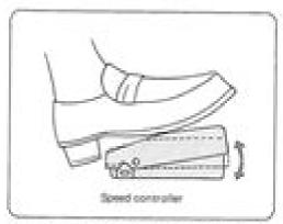
Sewing speed can be varied by the speed controller. The harder you press on the controller, the faster the machine runs.
